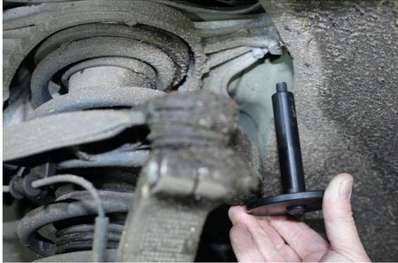
Install the FUCA (front upper control arm) ride height tool on to the mounting hole.
